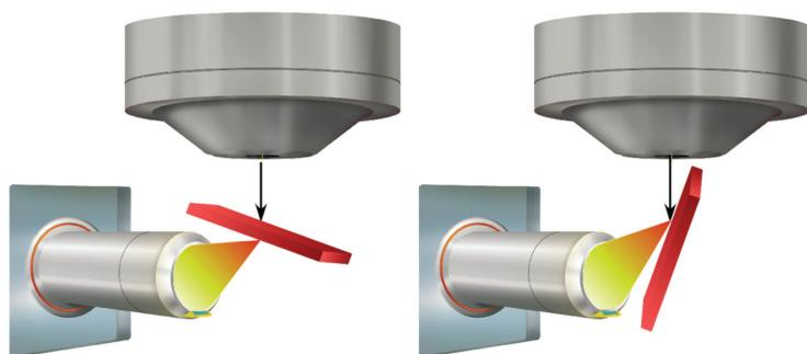
Figure 1. Schematics of t-EBSD (left) and standard EBSD (right).
