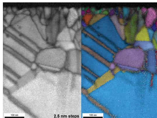
Figure 3. Image quality (left) and inverse pole figure (right) of a t-EBSD scan of Cu using a 2.5 nm step size.
