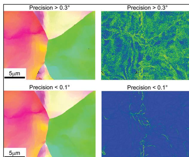
Figure 1. Standard Inverse Pole Figure (IPF) and KAM orientation maps at  $>0.3^\circ$
