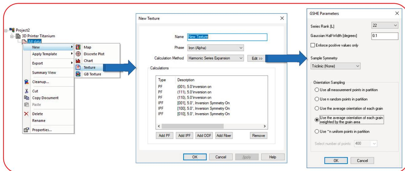
Figure 1. The Texture option in OIM Analysis™ where you can set GSHE parameters.
