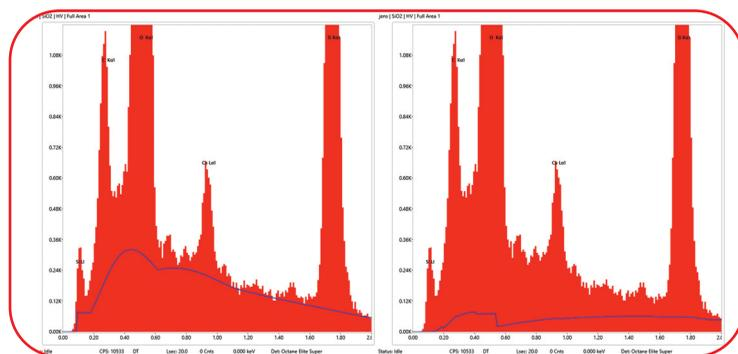
Figure 2. Example of SNIP method (left) and Bremsstrahlung model (right) on the same spectrum.
