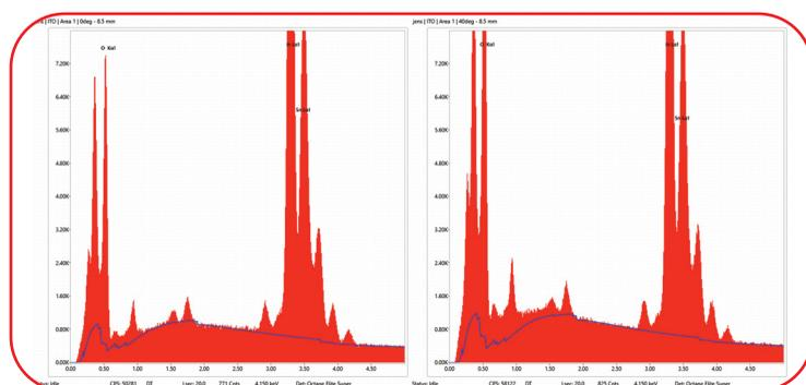
Figure 3. Spectra from an ITO sample where the left spectrum was collected with the stage flat while the stage was tilted towards the detector in the right spectrum. The background model was calculated for a flat sample in both spectra.
