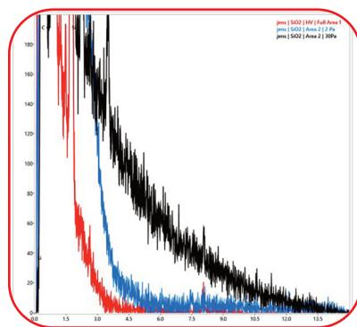
Figure 1. Quartz spectra at 15 kV showing variations in landing energy depending on vacuum conditions high vacuum (red), 2 Pa (blue), 30 Pa (black).
