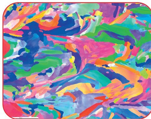
Figure 2. This is an EBSD IPF-Z image of SLM AM stainless steel.
