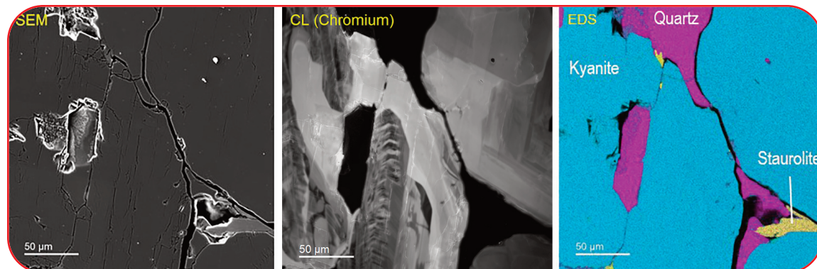
Figure 3. Co-acquired SEM (left), CL (center), and EDS (right) maps. EDS map indicates materials: quartz (magenta), kyanite (cyan), and staurolite (yellow).
