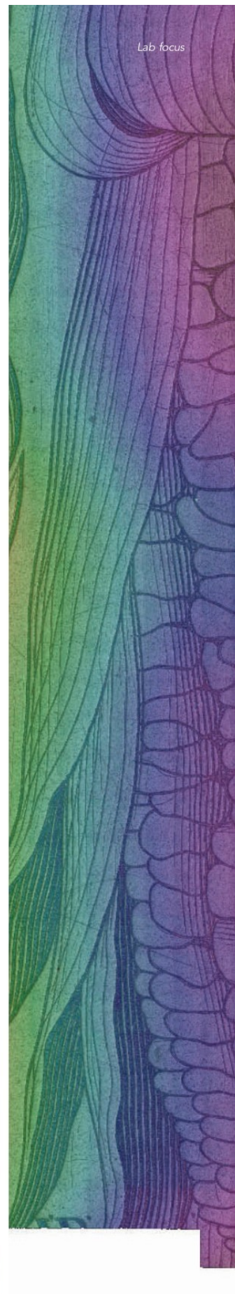
SWEETCORN from 17th century copper printing plate: When botanist, Robert Morison, created Praeludia Botanica in 1669 - including a huge collection of plants and herbs - he engraved a series of plant structures onto copper printing plates, which until a few years ago were thought to be lost. Now found, Dragnevski and colleagues used the Alicona profilometer to image the plates.
