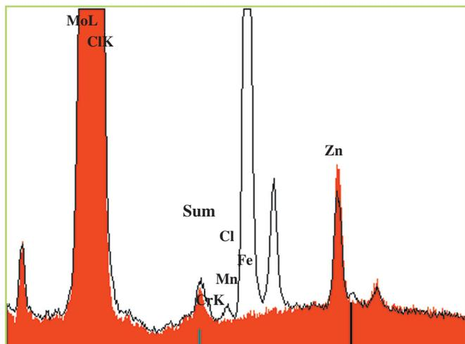
Figure 1. Comparison of spectra from inclusion and film.
