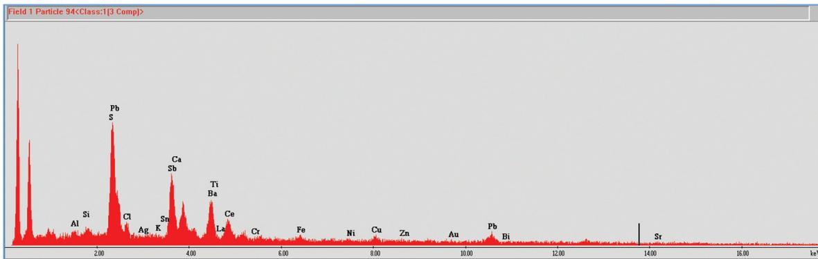
Figure 3 shows a spectrum collected in 1 second. Octane Elite yielded high input count rate (117 KCPS) and low dead time (26%) with a high output count rate of 86 KCPS with a 130 eV quality resolution, so there is high confidence in the statistical accuracy of the classified 3 component GSR particle.
