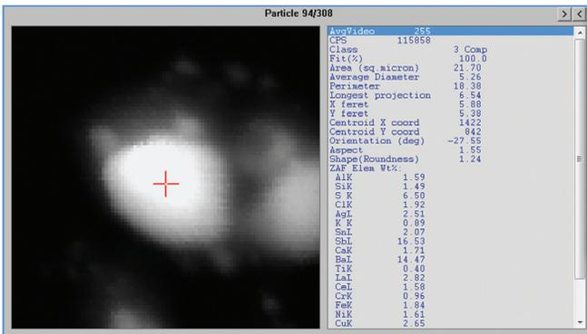
Figure 4 shows a zoomed in area of the 3 component particle that corresponds with the spectrum in Figure 3.
