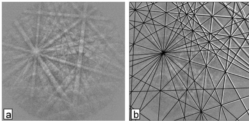
**Figure 1.** (a) Pattern from tetragonal zirconium oxide. (b) overlay of two potential indexing solutions to the pattern.
