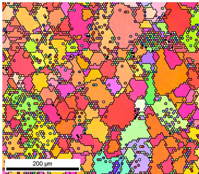
**Figure 2.** Orientation map from quartz without any post-processing.
