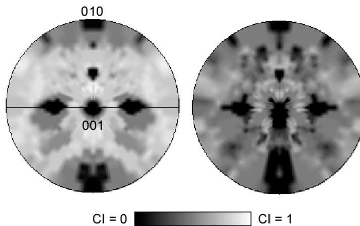
**Figure 3.** Stereographic projections showing the confidence index as a function of orientation for simulated patterns for zirconium oxide. These plots were generated assuming 6 bands were detected and using interplanar tolerance angles of (a) 3 degrees and (b) 6 degrees.
