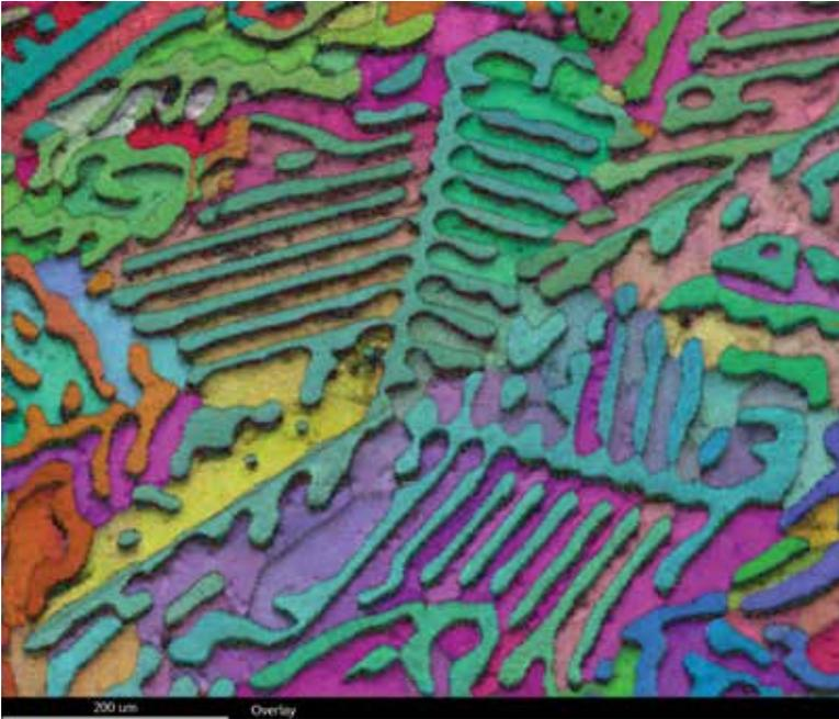
**Fig 3. Orientation map of an aluminum-germanium dual phase material**
