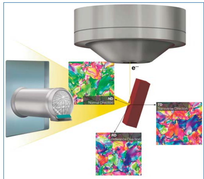
Schematic of EBSD detector, sample and electron beam geometries in SEM chamber.
