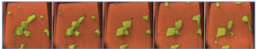
Figure 1. The typical 2D elemental maps of the primary elemental lines of a rare-earth modified steel sample.
